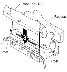
Figure 19 - Installing Front Log (#3)
